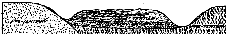
Fig. 1. Diagram showing occurrence of Tertiary formations in an old erosion valley. The surfaces at the extremes of the diagram represent an Eocene peneplain.
