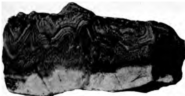
A—Fragment of vein showing crustification. A coarse phase. From New Republic mine. Actual size.
